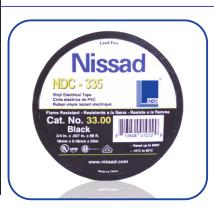
**Nissad NDC-335** is a 7mil (0.18mm) pressure sensitive PVC electrical insulation tape with high resistance to corrosion and various acids. It is flame retardant and can be used as primary insulation at not more than 600 volts.
